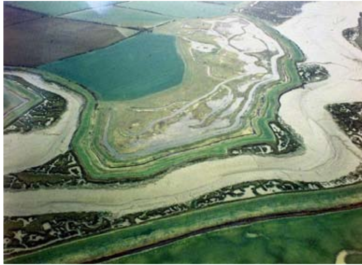
Figure 2: Abbots Hall realignment six months before the main breach in October 2002 (regulated tidal exchange in operation).
